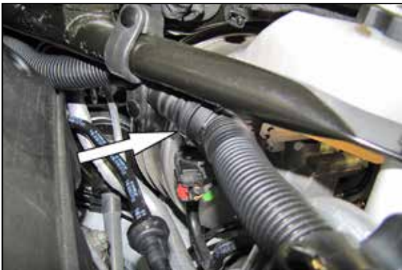
9. Disconnect the sound tube quick disconnect fitting and remove the complete sound tube system.
