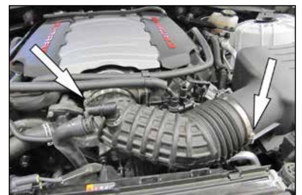
5. Loosen the hose clamps securing the intake tube to the throttle body and air filter housing and then remove the intake tube from the vehicle.
