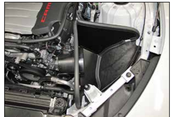
20. Install the K&N® heat shield assembly onto the air filter housing mounting grommets.
