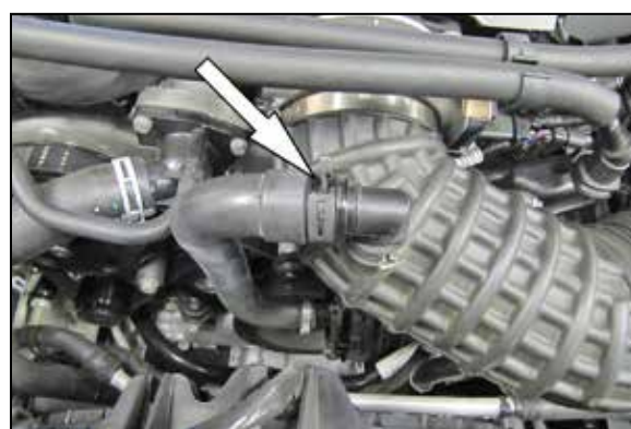
4. Release the spring clamp securing the sound tube to the fitting in the intake tube and then disconnect the sound tube.
