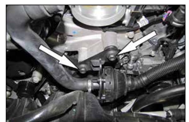
6. Remove the two bolts securing the sound drum to the front of the engine.
