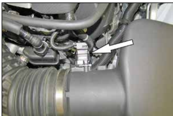
2. Disconnect the mass air sensor electrical connection.
